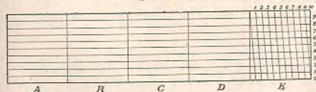
Illustrating the use of the protractor in measuring the distance between two points to ten places of decimals.
