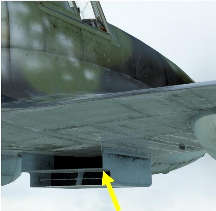
WATER RADIATOR OPEN
