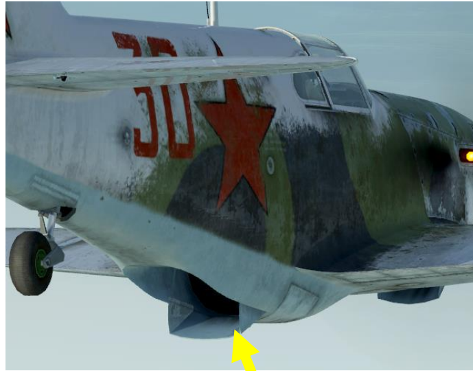
WATER RADIATOR OPEN
