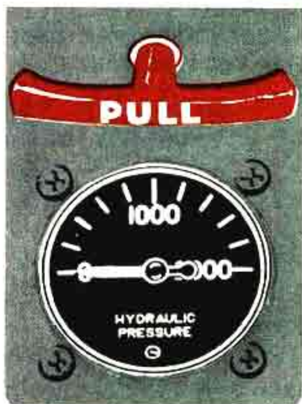
EMERGENCY HYDRAULIC RELEASE
