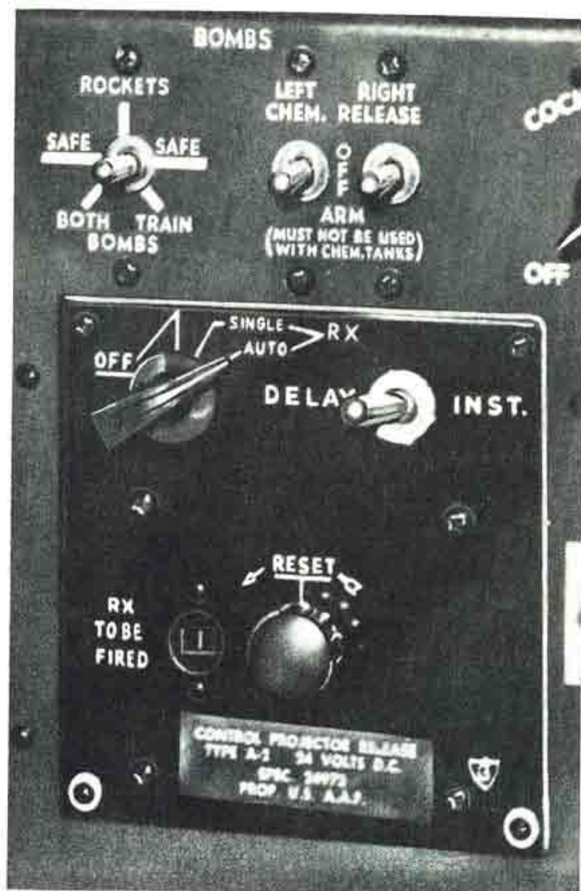
ROCKET CONTROL PANEL
